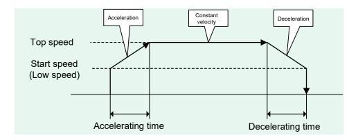
By setting the **start speed (Low speed), top speed, and acceleration time (Deceleration time),** CRUX performs internal calculation on the acceleration/deceleration rate and series of acceleration/deceleration operation are conducted automatically.
