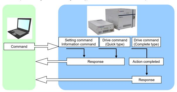
**Setting command** The commands as RST and WSY used for setting immediately return a response.
