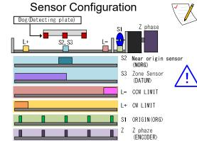
Based on the set origin return method, after moving near the specified sensor at the maximum speed of the specified speed table, it moves to the origin at the same speed with the starting speed of the speed table (Default: 500pps) and stops.
