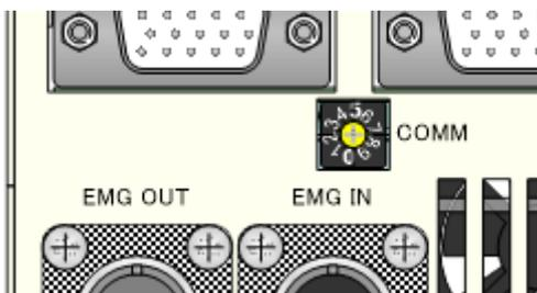
Rotary switch location for communication configuration of the CRUX-D
