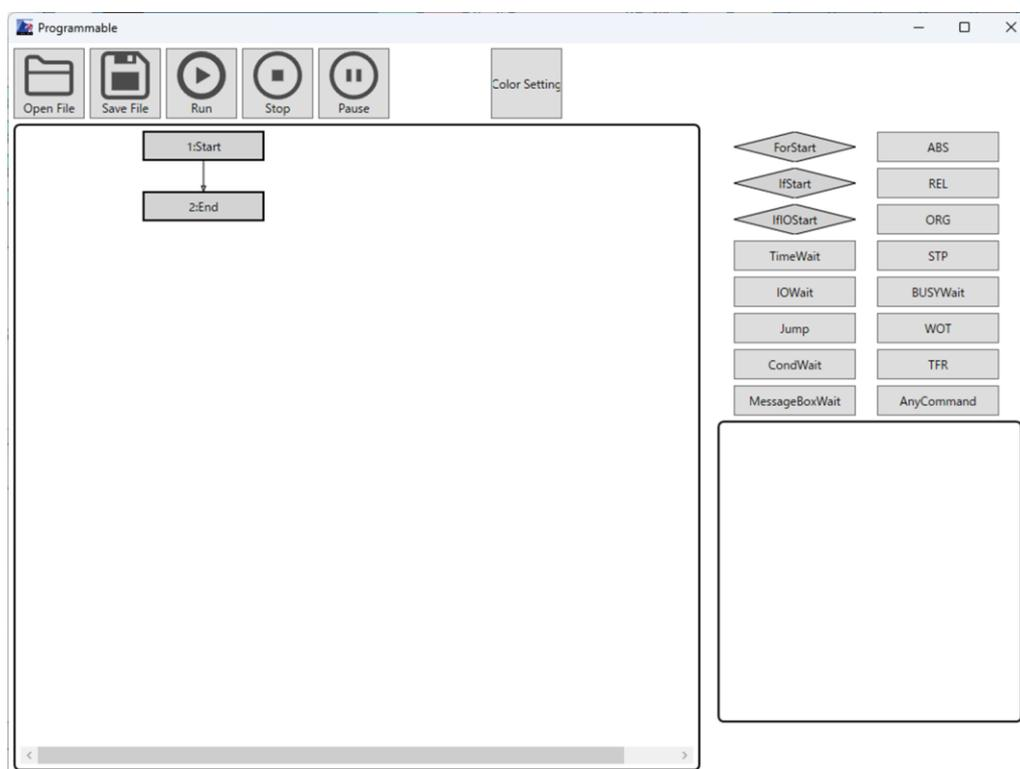
It automatically drives the stage connected to the controller according to the flowchart.
